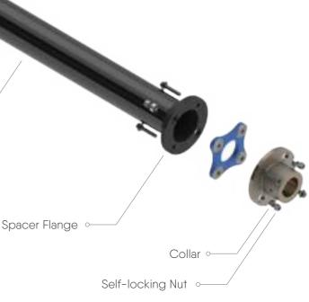
The spacer flange is entirely made out of composite material and its interface with the spacer has been developed to maximize the longevity of the coupling. Poor design of this interface is indeed a common cause for failure of composite couplings. During the ESCOFIL DFCT design and testing phase, ESCO put a special focus in optimizing the spacer-flange interface.
