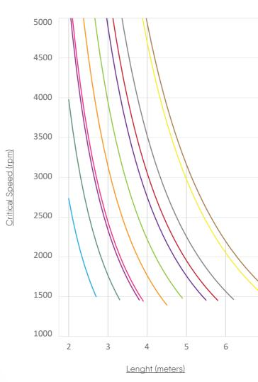
To be in line with guidelines of Cooling Tower Technology Institute, add an additional safety factor of 1.3 to determine the critical speed.
