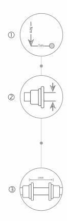
Select the size of ESCOFIL coupling that has the required torque capacity by comparing the figure in TABLE 2, Col. 2 (Max. continues Torque) with the figure obtained through to the following formula: T (Nm) =9550\*p\*Fu/n, with:
